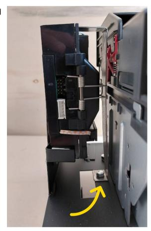
6. **Clear the upper coin path** by gently but firmly twisting the upper spring hinge (1) in the upwards direction.
