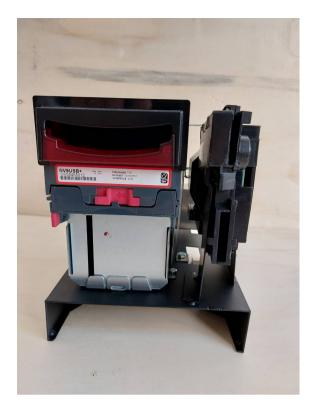
4. **Locate and loosen** but do not remove the screw located on the left side of the coin acceptor mounting bracket.
